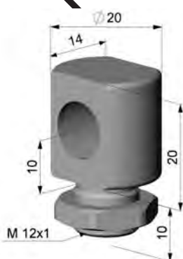
Mounting bolt with thread M 12x1, adjustable in one axis
