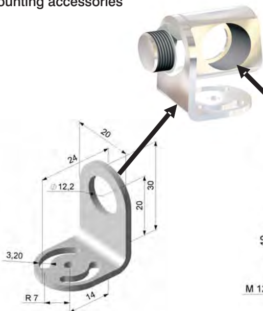
Mounting bracket, adjustable in one axis
