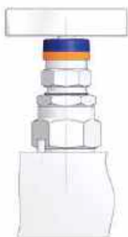
Color Coded Option FKM O-Ring Stem Seal with PCTFE Soft Tip
